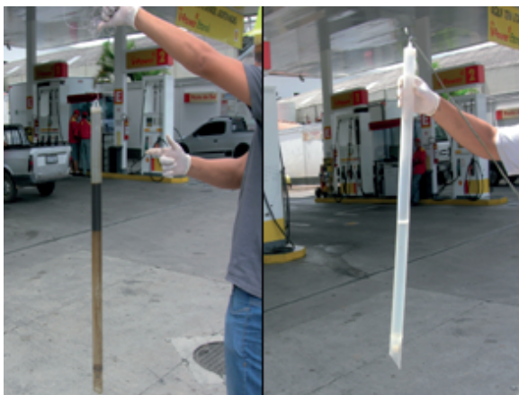
NAPL (Non-Aqueous Phase Liquid) before and 7 days after Redemtis/Fentox injection
